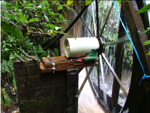
3m wheel cantilevered, directly connected to a 50:1 gearbox and Smart Drive PMA
