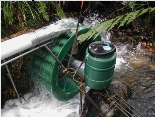
2m wheel cantilevered, connected to a 35:1 gearbox and Smart Drive PMA
