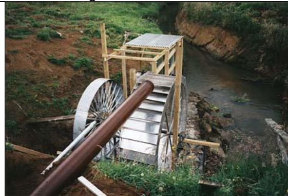
3.6m wheel mounted on two bearings, belt driven 2-stage gearing to a Smart Drive PMA
