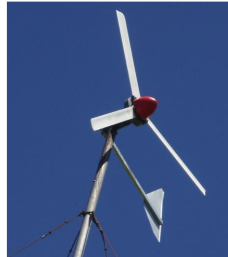
Smart Drive PMA on a Chinese turbine in strong winds
