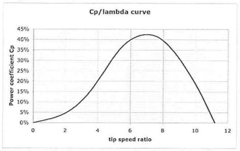
Cp peaks at the design tip speed ratio but it is still useful at lower and higher ratios, from about 5 to 9.
